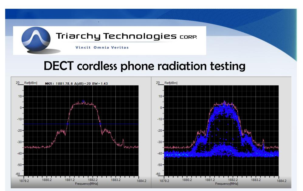
CH9=1881.792MHz, measured frequency is 1881.78MHz. Signal level is 6dBm, bandwidth is 1.43MHz.
