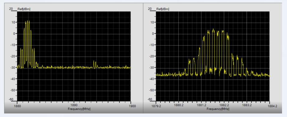
First find DECT signal at 20MHz SPAN, then change FREQ and SPAN setting to look around the detail the signal spectrum.
